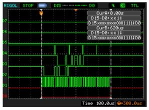
Fig. Example of a 5-Byte Digital Packet
